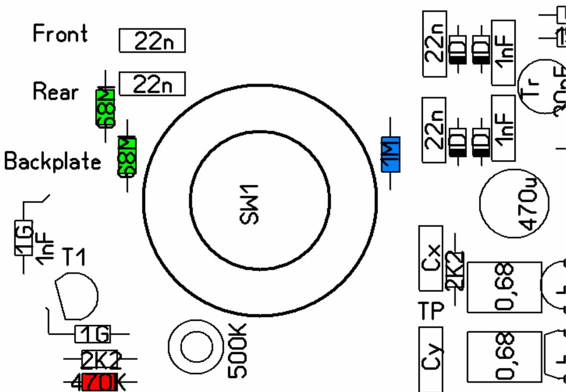
16. Place the 22 nF (.022uF) capacitors (red) and the 500 K.ohm trimpot. (blue).
