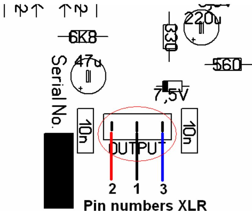
24. Connect the microphone circuit to a mixer or microphone amplifier with 48 V. Phantom power switched on, and check the voltage on the Test Point (TP). You measure between the connection going to pin 1 of the XLR, ('ground') and the TestPoint the arrow points at, so in fact one side of the 2.2 K.ohm resistor:
