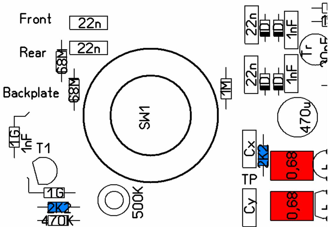
15. Next, insert the 470 K.ohm resistor (red), the 1 M.ohm resistor (blue) and the two 68 M.ohm resistors (green)
