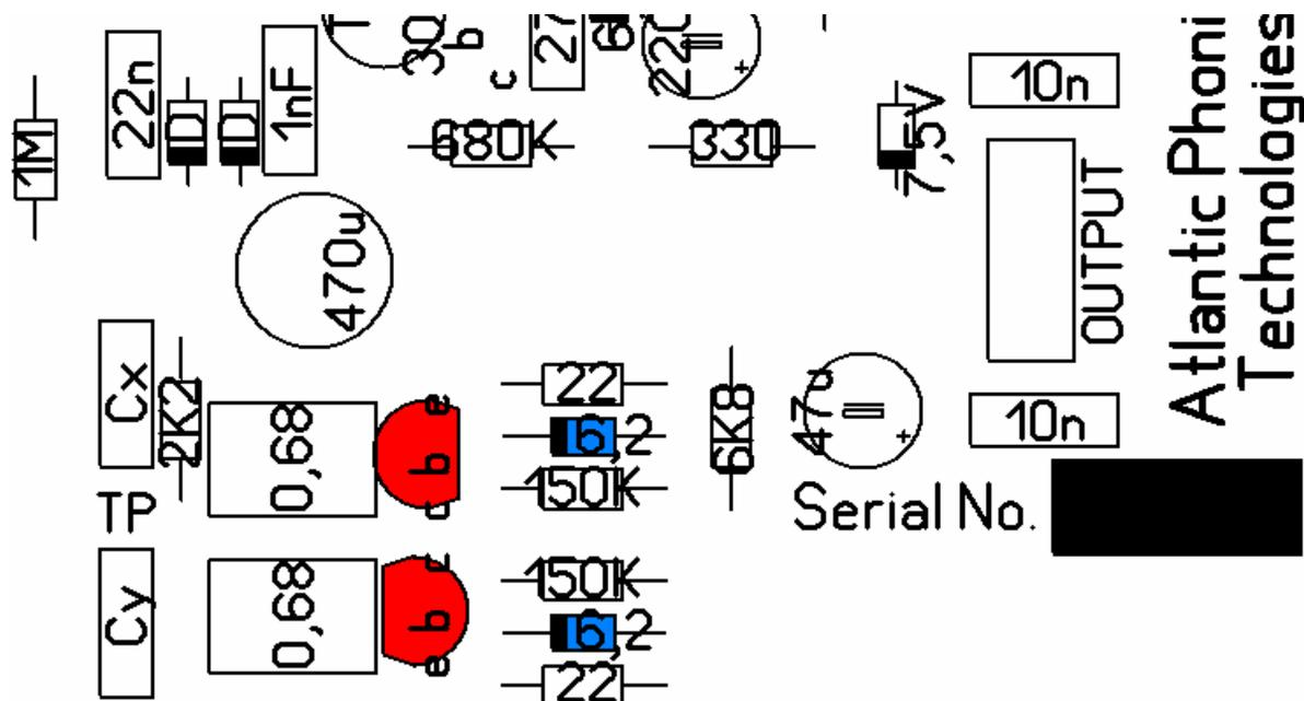
14. Now place the two 0.68 uF capacitors (red) and the two 2.2 K.ohm (2K2) resistors (blue)
