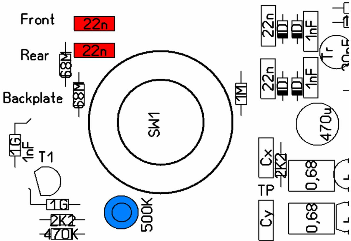
17. Now insert the two teflon insulator pins from the component side of the printed circuit board. They will serve as soldering points for the two 1 G.ohm resistors and the gate of the FET.
