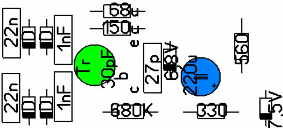
7. Place the BC547(b) transistor. The wires of the transistor are placed in a triangle, that matches the hole pattern of the printed circuit board. The flat side of the transistor should be close to the 27 pF capacitor.
