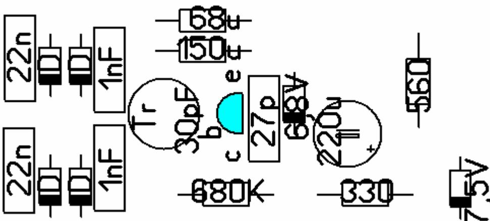
8. Last part in the DC/DC converter circuit is the 27 pF capacitor, marked 27.
