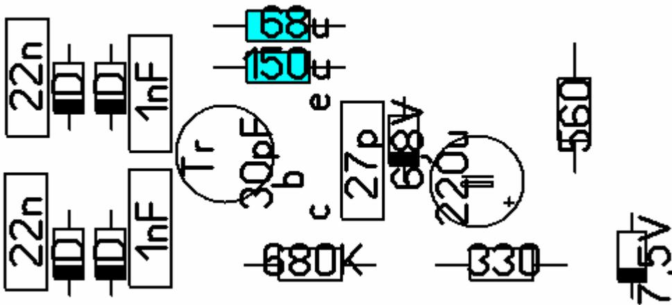
4. Now mount the next three resistors. 680K.ohm (**red**), 330 ohm (**blue**) and 560 ohm (**green**)
