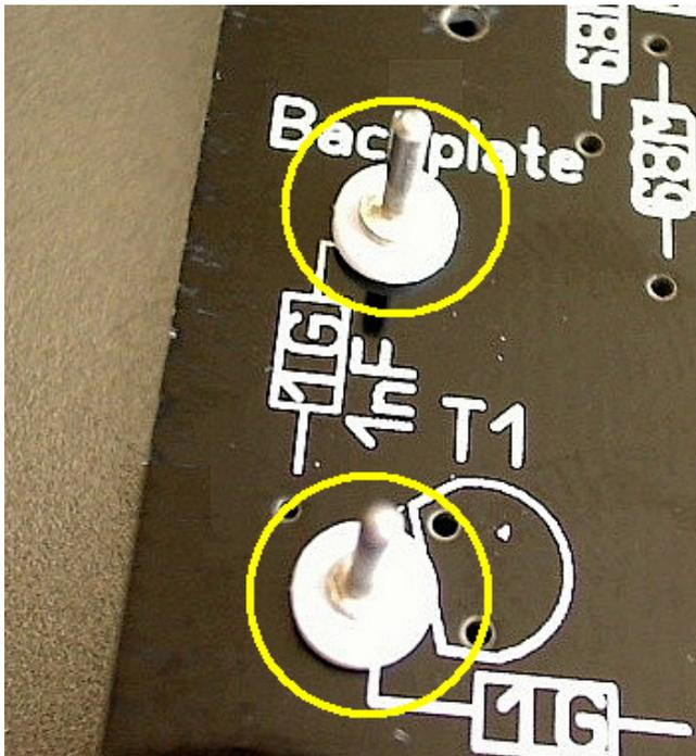
18. Prepare the (2SK170BL) FET, by bending the middle wire out, in the direction of the flat side with an angle of about 90 degrees. Insert the two outer wires of the FET as shown on the screenprint of the PCB. The wire in the middle, that we have just bent out, goes to the teflon insulator pin. Solder the outer wires of the FET to the PCB, but **don't** solder the wire yet to the teflon insulator pin!
