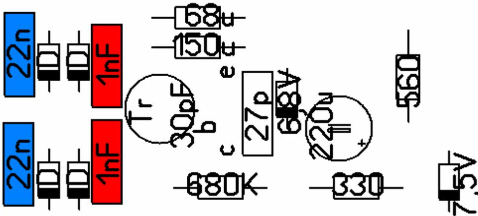
6. Insert the (green) 30 pF trimmer (**green**) and the 220 uF electrolytic capacitor (**blue**). Observe the polarity, the + side of the capacitor should be close to the 330 ohm resistor.
