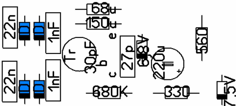
2. Next we mount the two other zener diodes, marked 6V8 and 7V5, respectively 6.8 Volt (**blue**) and 7.5 Volt (**red**). Here it is also important to observe the correct orientation!
