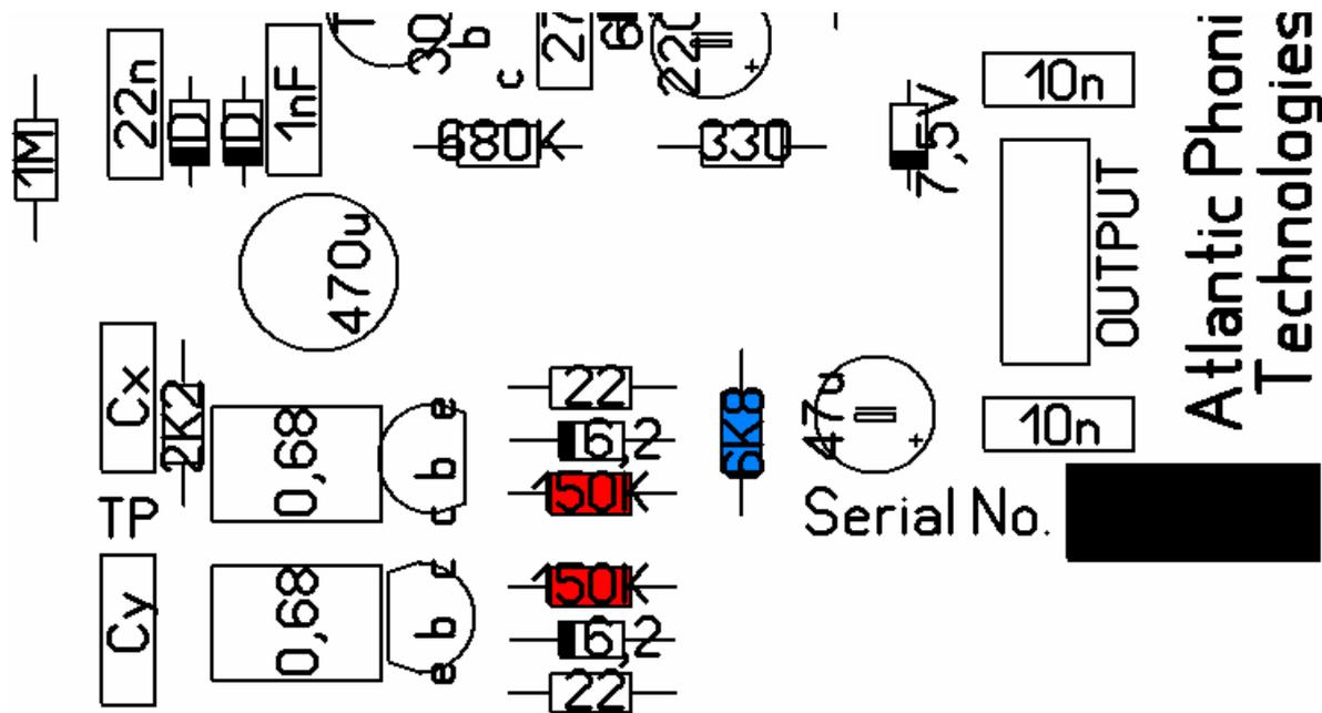
13. Now place the two BC557(b) transistors (**red**). This time the wires from the transistors are in a single row. Note that the flat side of the transistors is on the left for the bottom one, and to the right for the top one. Also place the two 6.2 V. (6V2) zener diodes (**blue**).
