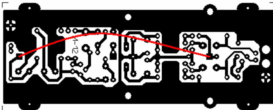
The wire should make a connection between the two square pads. Don't forget this, otherwise the microphone won't work!
