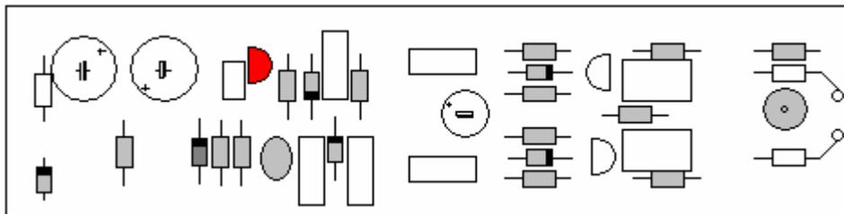
Now we put in the two BC557B transistors. The holes are on a single row now. Observe how the transistors should be placed, the flat side is on the right side for the upper one, and on the left side for the lower one.
