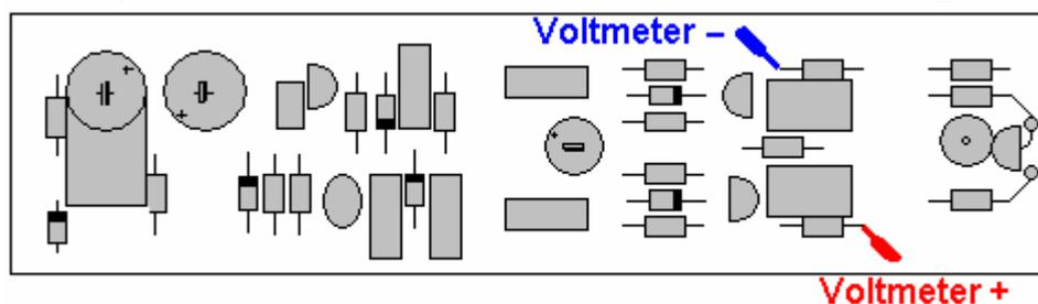
Adjust the cermet trimmer potentiometer for a voltage of 5.25 Volts.
