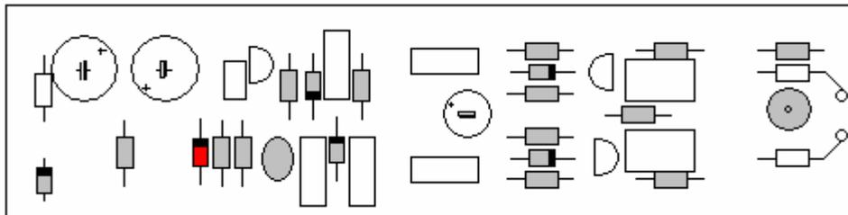
Now we place the BC547B transistor. The wires are in a triangle that fits the hole pattern in the PCB:
