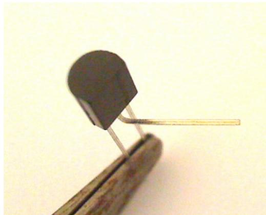
Now we insert the FET in the two holes near the small edge of the PCB and solder it into the circuit. The leg that we have just have bent, goes to the teflon feedthrough:
