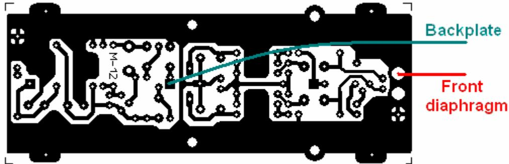
The front diaphragm is connected to the teflon feedthrough as is shown above. This works fine if you have a single sided capsule, or if you have a double sided capsule and you want to make a cardioid microphone. In this case leave the wire from the back diaphragm floating. Don't cut it off!!! Now you can always use the back diaphragm later, in case the front diaphragm becomes damaged or polluted.
