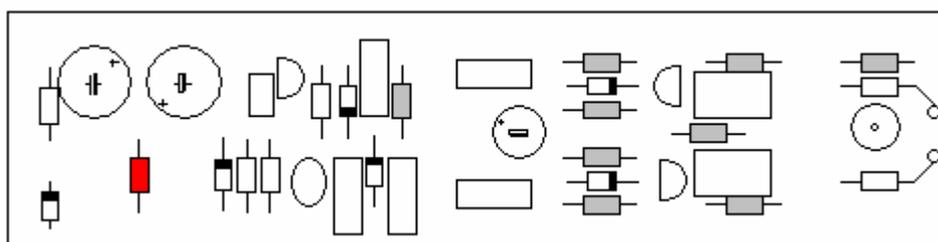
Insert the 680 K.Ohms resistor in this position
