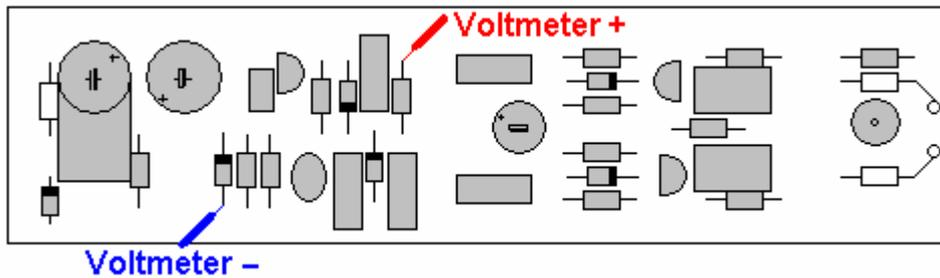
If the voltage is lower than 60 Volts, turn the trimmer capacitor so that the rotor blades are more between the stator blades. (=Clockwise)
