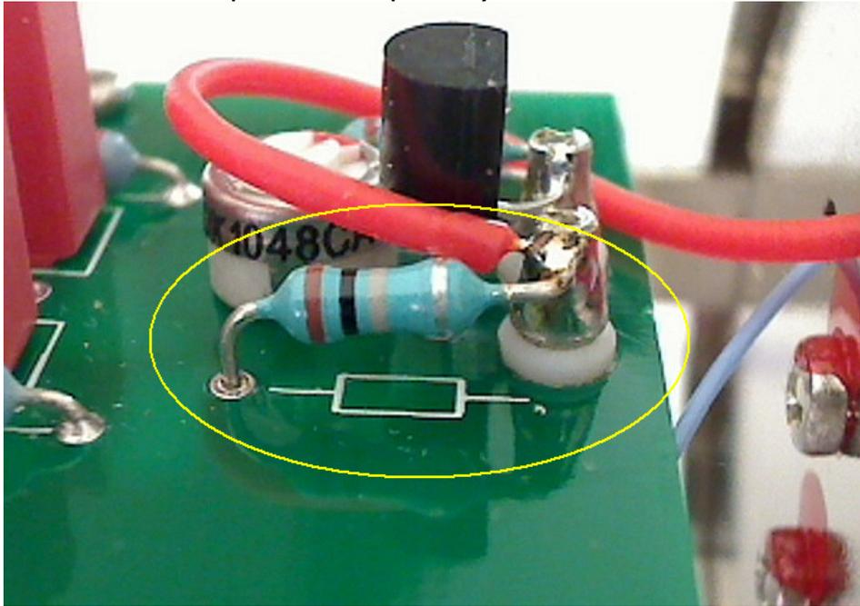
Next, we install the FET. First we bend the wire in the middle outwards, under an angle of about 90 degrees in the direction of the flat side of the black body.
