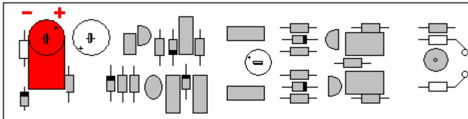
Next we put in the 220  $\mu\text{F}$ . Also here, polarity is important!
