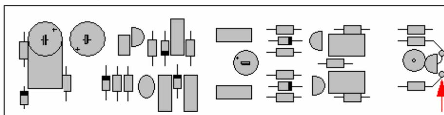
Slowly increase the level of the tone generator and observe the output signal (pin 2 or 3 on the XLR connector). Adjust the trimmer potentiometer for symmetrical clipping on both output pins.
