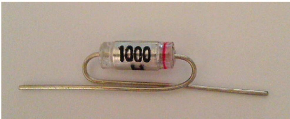
Then bend the wires of the styroflex capacitor under an angle of 90 degrees and cut the wires to length.
