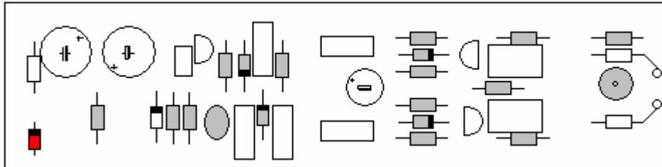
The last diode we place is the 6.8 V. Zener diode. Same procedure as with the others.
