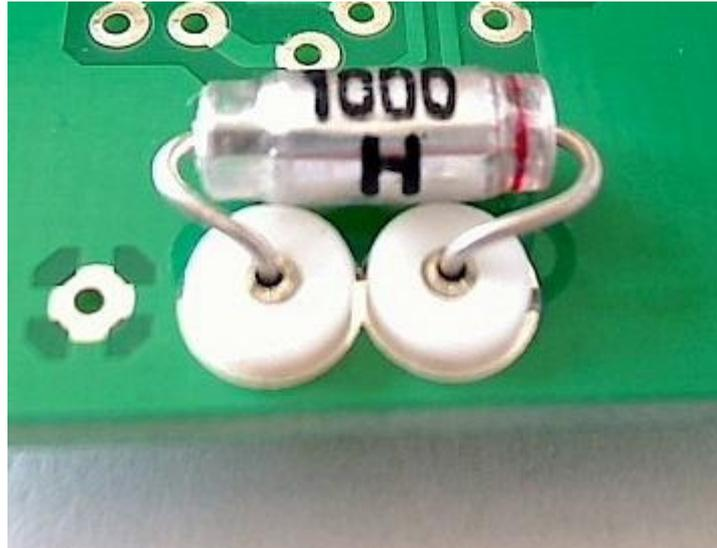
The styroflex capacitors are sensitive to overheating. It might be a good idea to place an alligator clip on the wire of the capacitor close to the capacitor body while soldering. This way the heat is absorbed.
