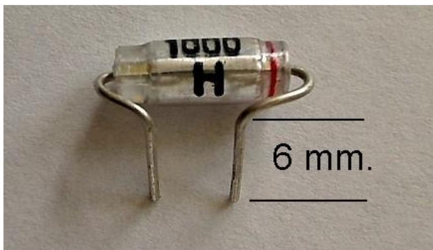
Insert the wires of the styroflex capacitor in the holes of the teflon feedthroughs from the trace side of the PCB. The length is correct if the wires of the 1 G.ohm resistors on the component side are just touched. Now solder all wires connected to the teflon feedthroughs.
