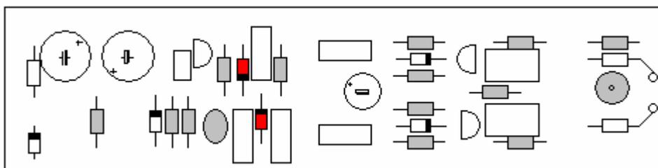
Take care that the black ring on the diode matches the white line on the PCB!
