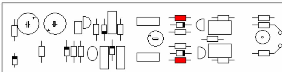
The components we have to place are marked with a red color. During the next step, the components already on the board will be displayed with a gray color.
