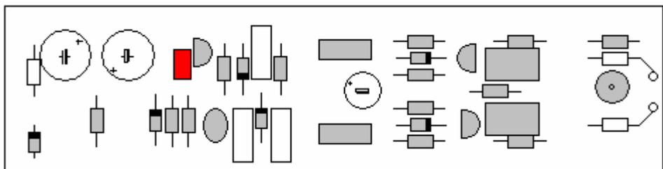
The next step is to put the 1 nF capacitor here:
