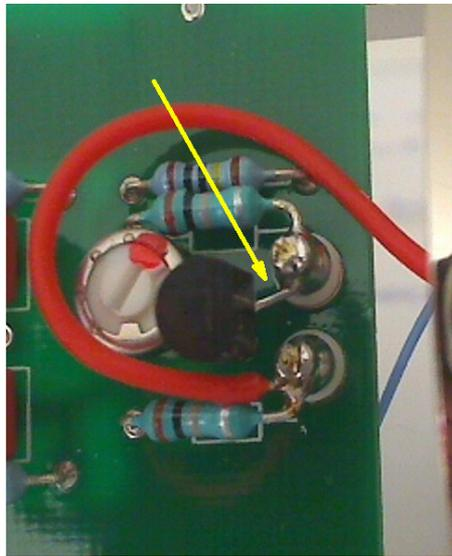
Now we take the 1 nF styroflex capacitor and fold the two wires close to the body of the capacitor, like this.
